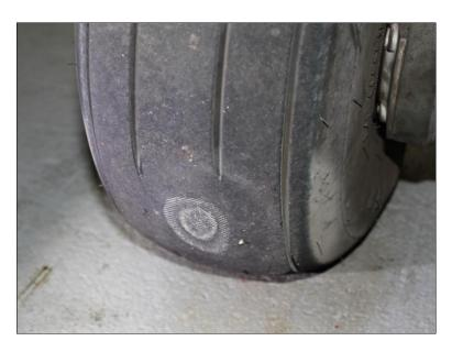
Photo No. 2: Flat spot on right main tyre
