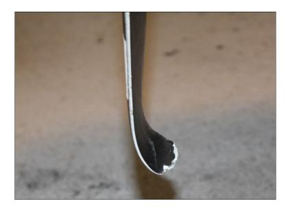
Photo No. 1: Detail of damage to one of the left propeller blades
